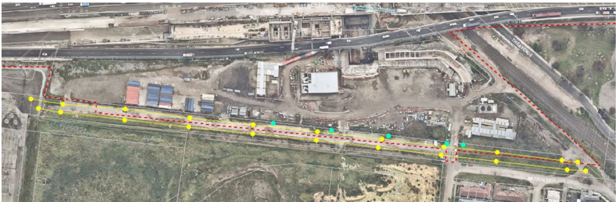
Figure 1: Plan showing 22 new HV poles and wires in Ausnet easement (yellow dots)
